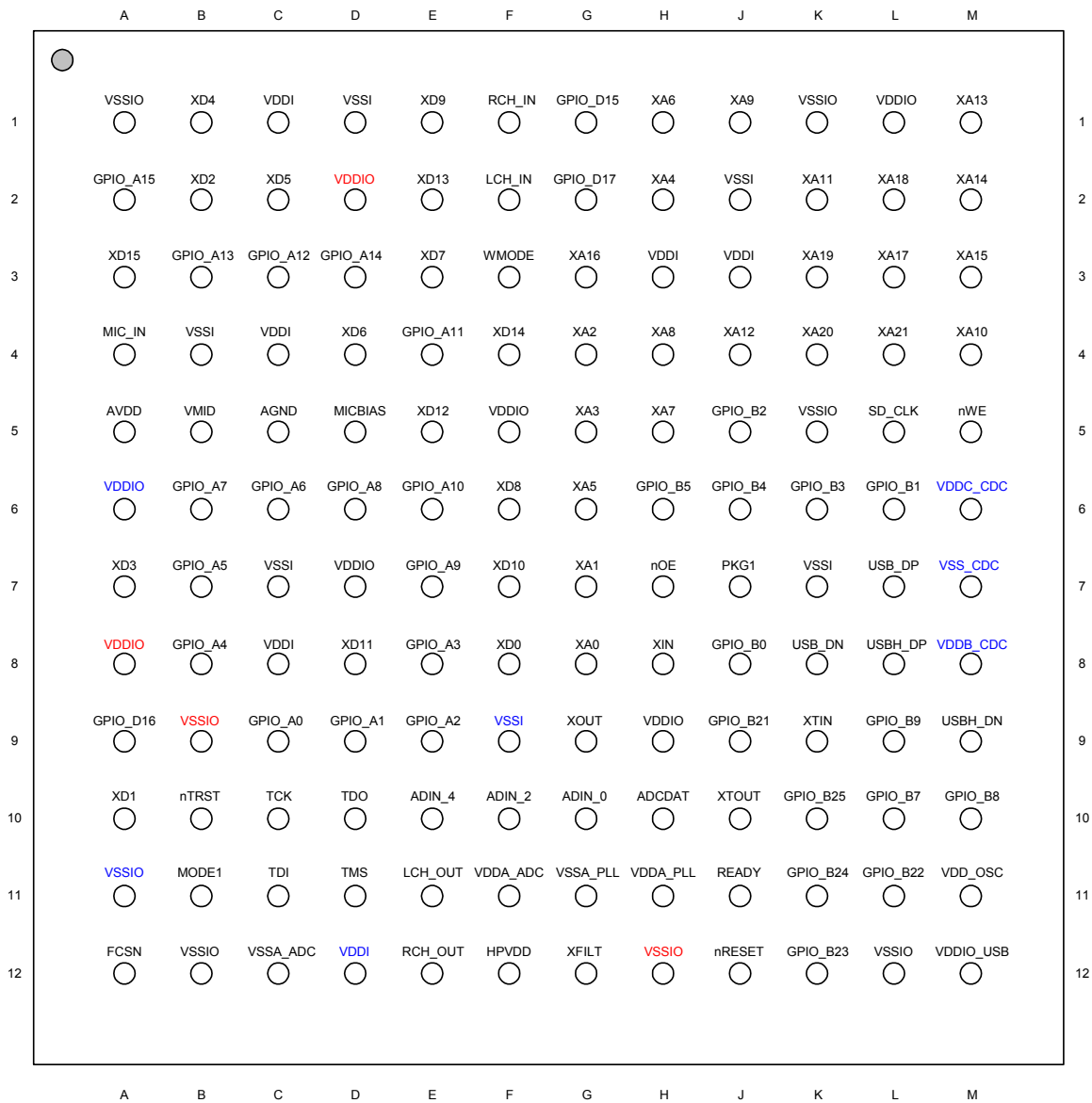
Figure 1.14 TCC768 Package Diagram (144-BGA-1010 / Bottom View)
