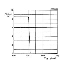
$\label{eq:fig.4} Fig. 4 \quad \text{Keyed AGC output voltage V}_{20} \text{ as a function} \\ \text{of input voltage V}_{14}. \text{ Measured in test circuit} \\ \text{Fig. 1 at V}_3 = 2 \text{ V; I}_{20} = 0.$
