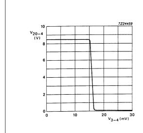
Fig.3 Keyed AGC output voltage  $V_{20}$  as a function of RMS input voltage  $V_3$ . Measured in test circuit Fig.1 at  $V_{14} = 0.7 \text{ V}$ ;  $I_{20} = 0$ .
