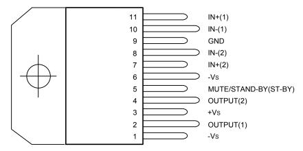
\* TAB CONNECTED TO PIN 6
