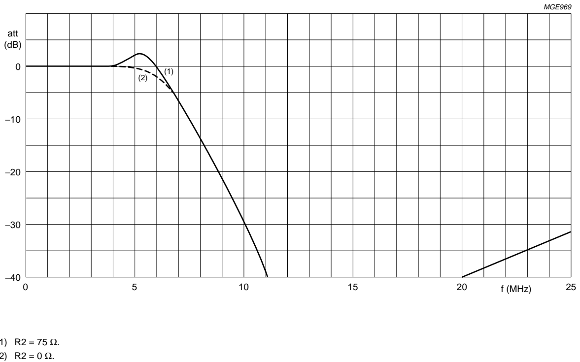
Fig.9 Frequency response for filter shown in Fig.8.
