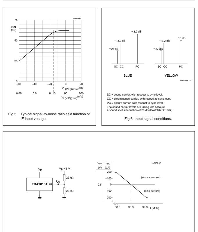
Fig.7 Measurement conditions and typical AFC characteristic.
