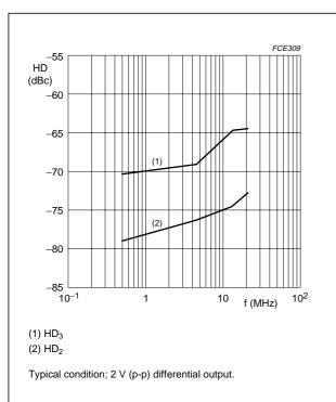
Fig.8 Harmonic distortion as a function of frequency for minimum gain plus 12 dB.
