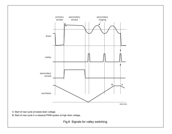
As soon as the oscillator voltage is high again and the secondary stroke has ended, the circuit waits for the lowest drain voltage before starting a new primary stroke. This method is called valley detection. Figure 8 shows the drain voltage together with the valley signal, the signal indicating the secondary stroke and the oscillator signal.
