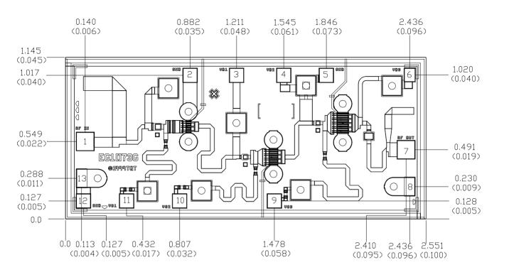
Units: millimeters (inches) Thickness: 0.1016 (0.004)
