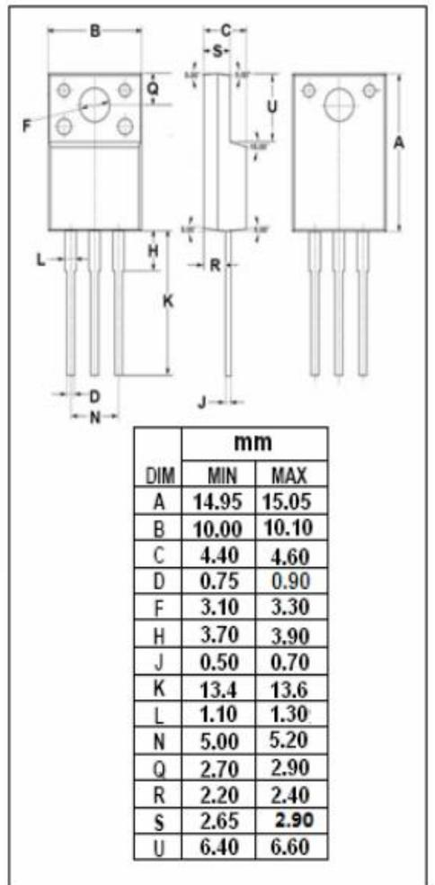
**Isc N-Channel MOSFET Transistor**
