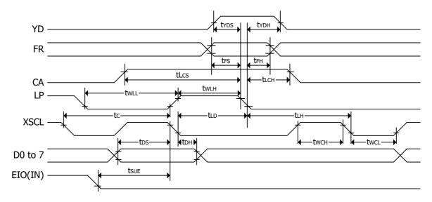
$\text{VSS} = -3.3 \text{ V} \pm 0.3 \text{ V}, \text{ VIH} = 0.2 \text{ VSS}, \text{ VIL} = 0.8 \text{ VSS}$
