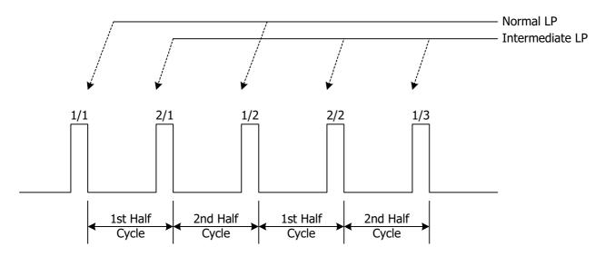
The segment output voltage during 1/2 H operation also follows the display data of 4.3 and the diagram showing the relationship between the LC AC signal FR and the segment output voltage. In the signal B/ A that indicates the number of the LP, the "A" in the figure indicates LP during a normal drive, and "B" differentiates between the normal LP and the intermediate LP (where B = 1 is normal and B = 2 is intermediate).
