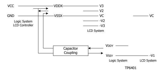
When the TP6410 and TP6401 are used to structure an extremely low-power module system, the power supplies for the TP6410 logic systems and LCD systems, and the power supplies for the LCD controller should have the voltage relationships shown in the figure above.
