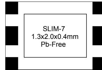
6-pin 1.3 x 2.0 x 0.4 mm SLP Package
