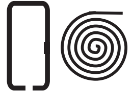
Figure 30: Loop or Trace Antenna
