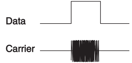
Figure 12: CPCA (AM) Modulation
