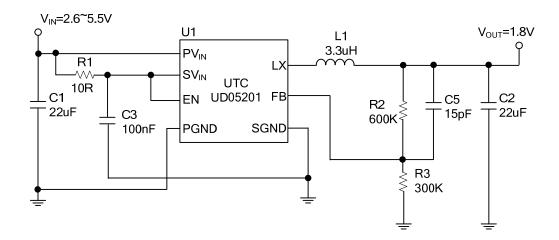
$V_{OUT}$ =0.6 × (1+R2/R3) R2=510K $^{\sim}$ 820K
