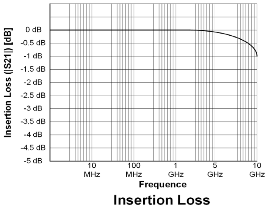
Figure 5. Typic Insertion Loss vs. Freqence
