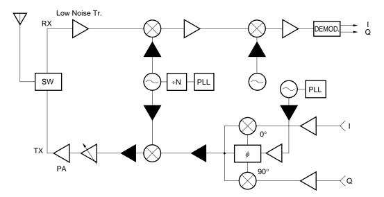
These ICs can be added to your system around  $\blacktriangle$  parts, when you need more isolation or gain. The application herein, however, shows only examples, therefore the application can depend on your kit evaluation.
