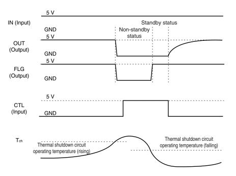
While the thermal shutdown circuit is activated, the output pins are in the OFF status. However, the IC does not enter the standby status even if all the CLT pins are deasserted inactive at the same time.
