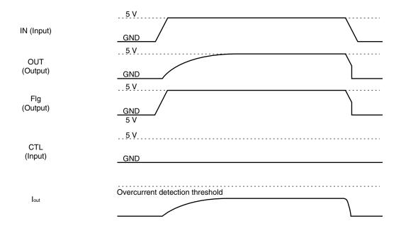
If the CTL signal is asserted active after power has been turned ON, OUT executes the soft-start operation (output transition time: 8 ms MAX.). In addition, FLG output is fixed to "L" if the supply voltage is lower than the operating voltage of the undervoltage lockout circuit (UVLO) on power application.
