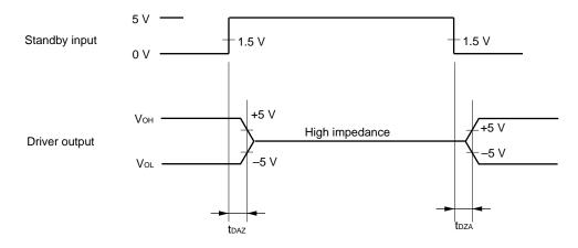
Do not perform communication within the standby output transition time tDZA on power application or on releasing the standby mode.
