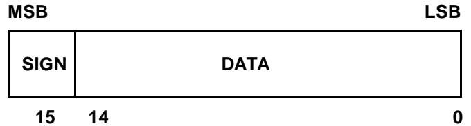
Figure 31a. Single 16-bit Precision Fixed-Point Data
