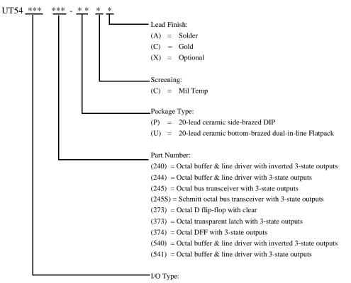
(ACS) = CMOS compatible I/O level (ACTS) = TTL compatible I/O level
