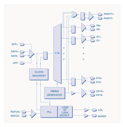
The VSC8171 mux offers integration of a high output swing mux with a lowjitter generation clock multiplier unit. The VSC8172 demux offers an integrated limiting amplifier, demux and high jitter tolerant clock and data recovery unit. Vitesse has eyes for you: "The best data eyes in the business."
