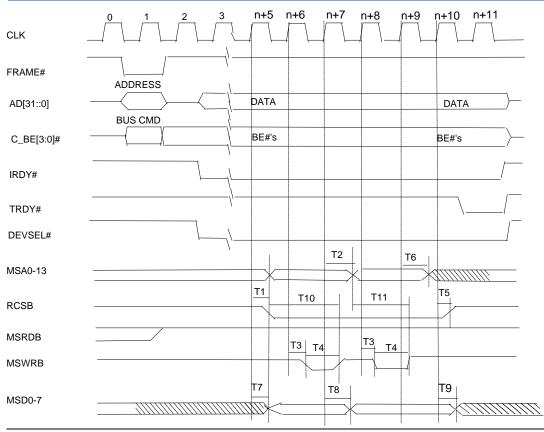
Note: 1) The other timing requirements for PCI signal are as the read transaction timing.
