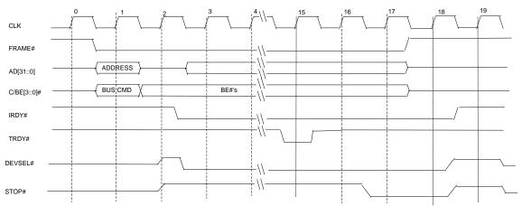
Because W89C940 don't support memory command in burst mode. When the host try to send memory command in burst mode, the first data phase is completed. TRDY# and IRDY# are deasserted, but the FRAME# is asserted for the next data phase. The device will assert STOP# to terminate the transaction. Data is not transferred after STOP# is asserted. The host need to initiate another transaction for further data transfer. The timing is shown above.
