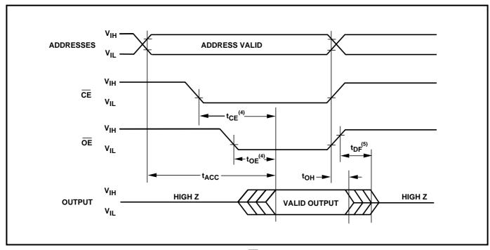
**NOTE:** 4.  $\overline{OE}$  may be delayed up to  $t_{CE} - t_{OE}$  after the falling edge of  $\overline{CE}$  without impact on  $t_{CE}$ .
