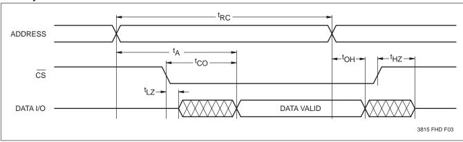
Note: (6)  $t_{LZ}$  min. and  $t_{HZ}$  min. are periodically sampled and not 100% tested.
