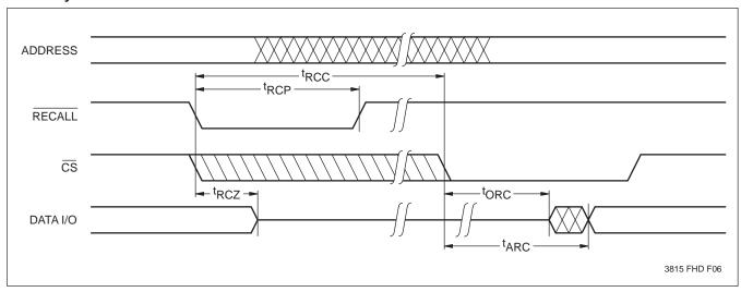
Note: (7)  $\overline{\text{Recall}}$  rise time must be less than 1 $\mu$ s.
