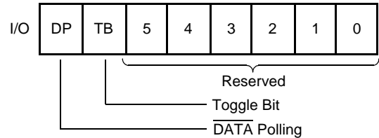
Figure 1. Status Bit Assignment
