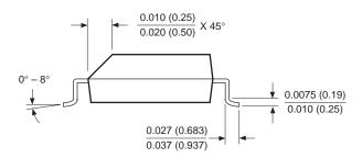
NOTE: ALL DIMENSIONS IN INCHES (IN PARENTHESIS IN MILLIMETERS)
