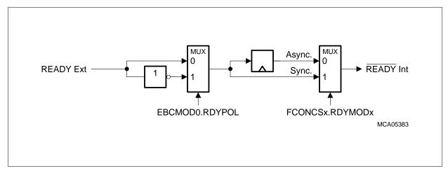
Figure 9-11 External to Internal READY Conversion
