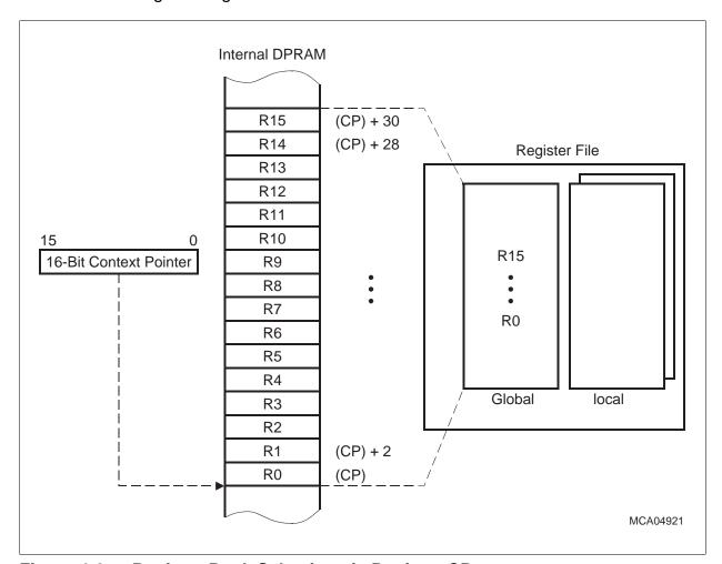
Figure 4-6 Register Bank Selection via Register CP
