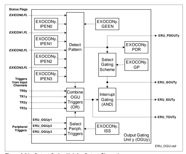
Figure 6-24 Output Gating Unit for Output Channel y
