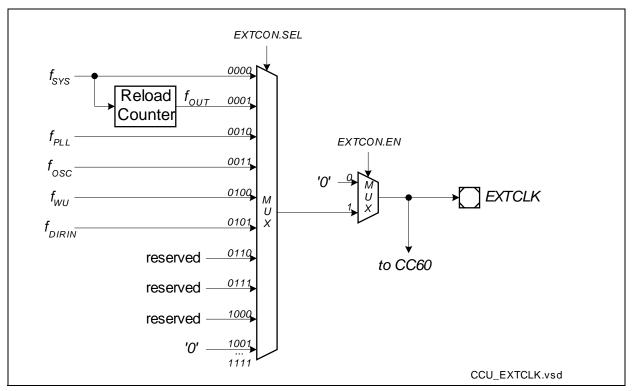
Figure 6-13 Clock Control Unit, EXTCLK Generation
