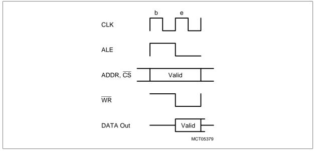
Figure 9-7 Fastest Write Cycle Demultiplexed Bus
