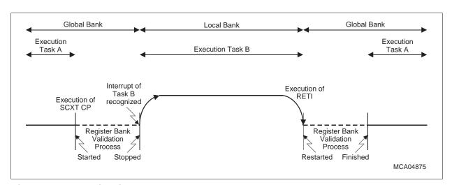
Figure 4-10 Validation Process Interrupted by Local-Bank Interrupt
