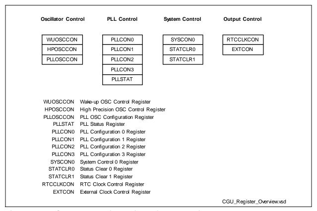
Figure 6-2 Clock Generation Unit Register Overview
