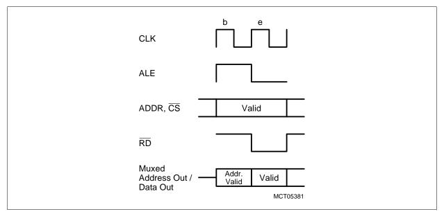
Figure 9-9 Fastest Write Cycle Multiplexed Bus
