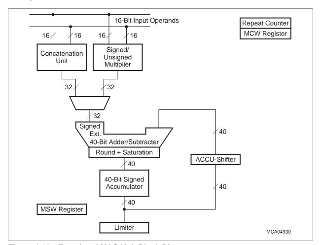
Figure 4-18 Functional MAC Unit Block Diagram
