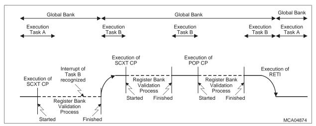
Figure 4-9 Validation Process Interrupted by Global-Bank Interrupt
