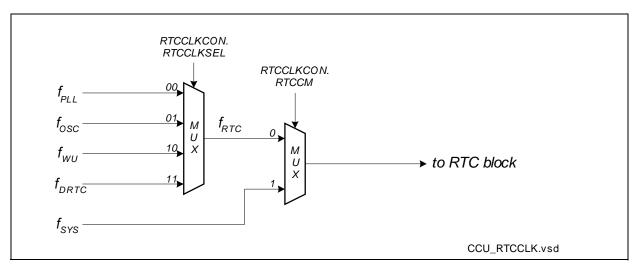
Figure 6-12 Clock Control Unit, RTCCLK Generation
