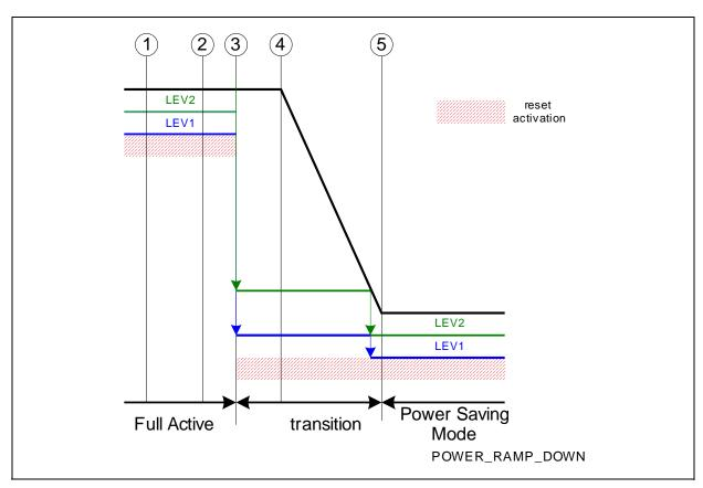
Figure 6-28 Ramp-down Example
