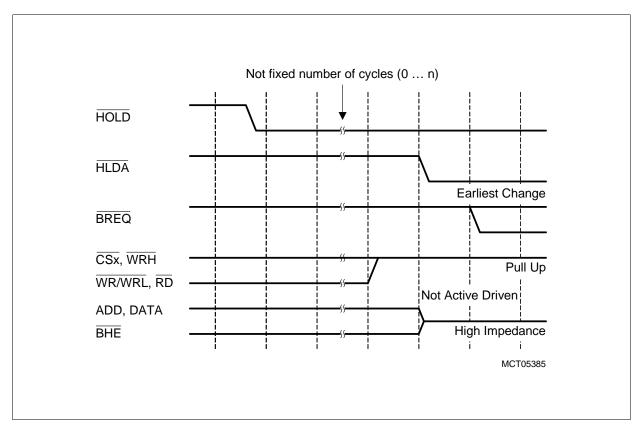
Figure 9-13 Releasing the Bus by the Arbitration Master
