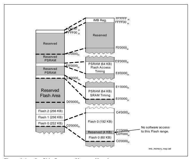
Figure 3-4 On-Chip Program Memory Mapping
