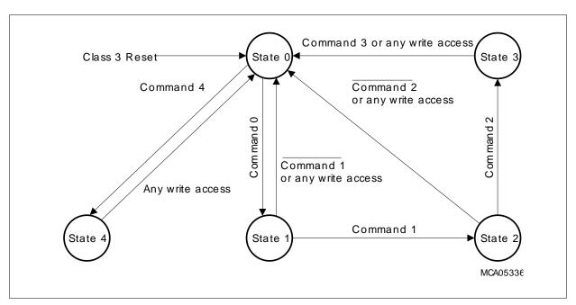
Figure 6-35 State Machine for Security Level Controlling
