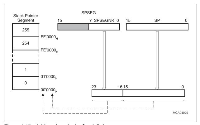
Figure 4-17 Addressing via the Stack Pointer
