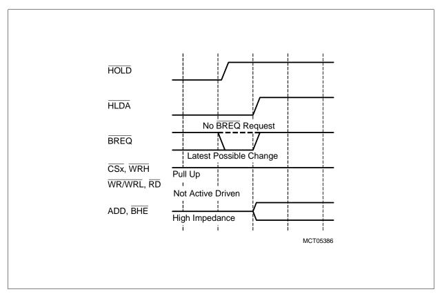
Figure 9-14 Regaining the Bus by the Arbitration Master
