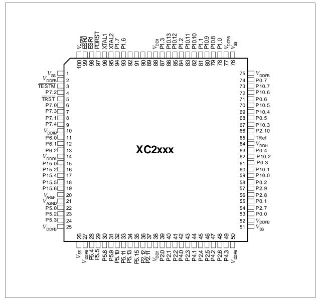
Figure 13-2 Pin Configuration PG-LQFP-100 Package (top view)
