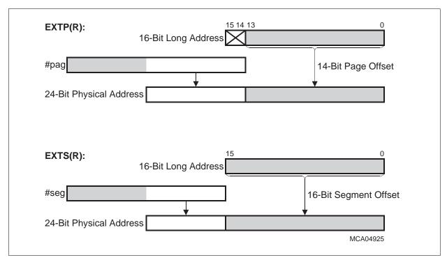
Figure 4-14 Overriding the DPP Mechanism
