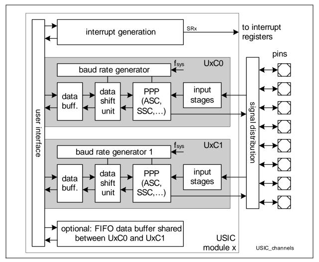
Figure 2-3 Channel Structure
