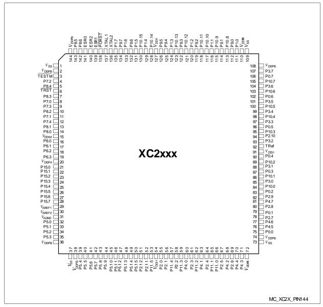
Figure 13-1 Pin Configuration PG-LQFP-144 Package (top view)
