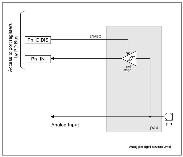
Figure 7-3 Structure of Port 5 and Port 15
