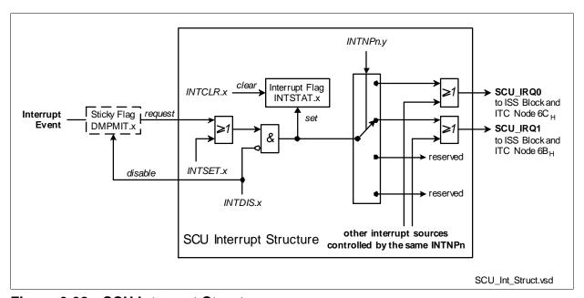
Figure 6-38 SCU Interrupt Structure
