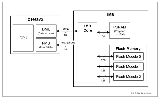
Figure 3-9 IMB Block Diagram
