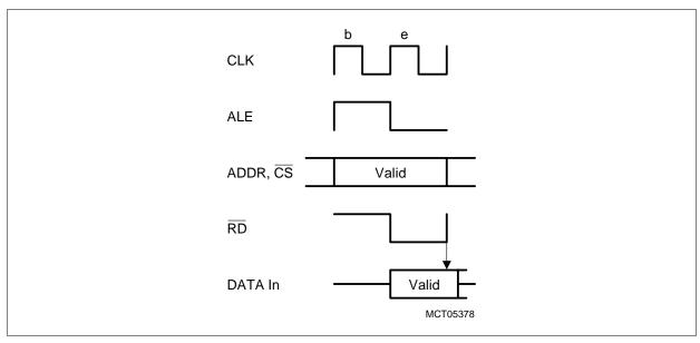
Figure 9-6 Fastest Read Cycle Demultiplexed Bus
