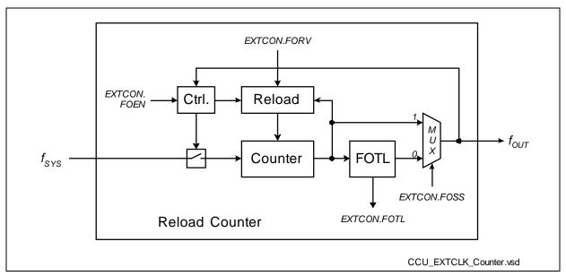
Figure 6-14 Programmable Frequency Output Generation
