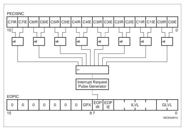
Figure 5-4 End of PEC Interrupt Sub Node
