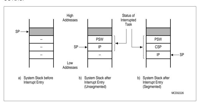
Figure 5-5 Task Status Saved on the System Stack
