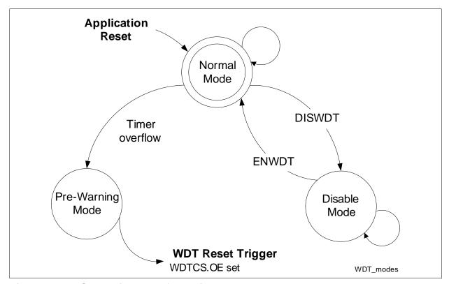
Figure 6-32 State Diagram of the Timer Modes
