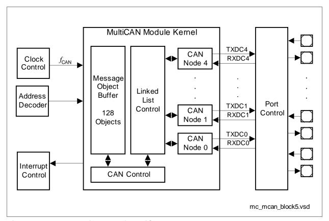
Figure 2-4 Block Diagram of MultiCAN Module
