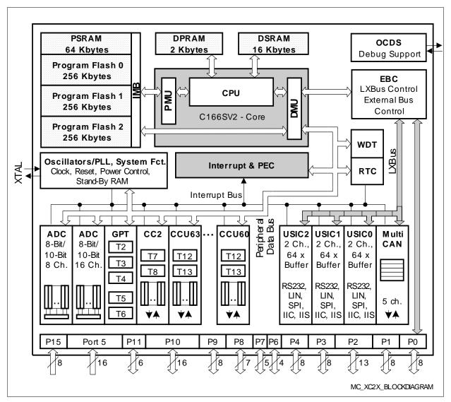
Figure 2-1 XC2000 Functional Block Diagram
