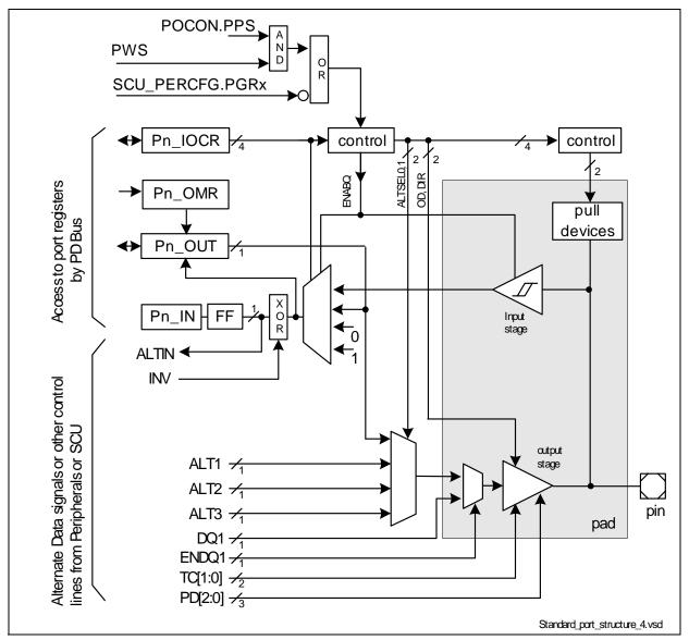
Figure 7-1 Structure of the Ports without Hardware Override Functionality
