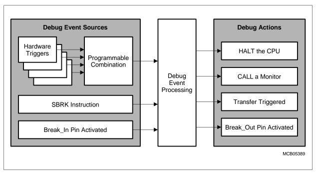
Figure 11-2 OCDS Concept: Block Diagram
