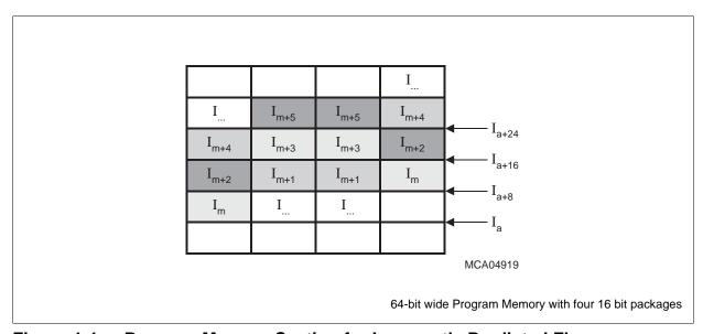
Figure 4-4 Program Memory Section for Incorrectly Predicted Flow
