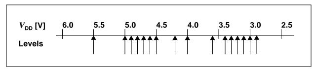
Figure 6-27 Threshold Levels for Supply Voltage Supervision by SWD
