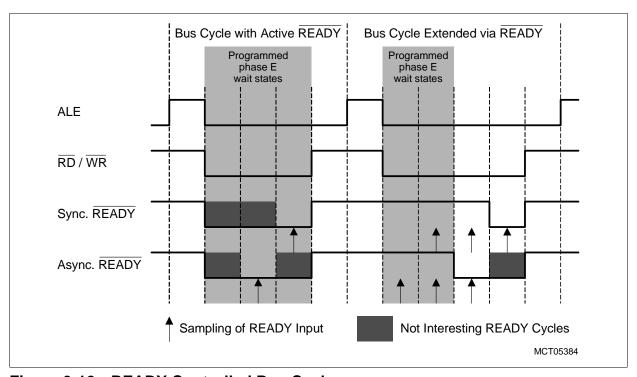
Figure 9-12 READY Controlled Bus Cycles
