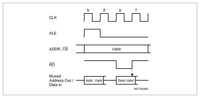
Figure 9-8 Fastest Read Cycle Multiplexed Bus
