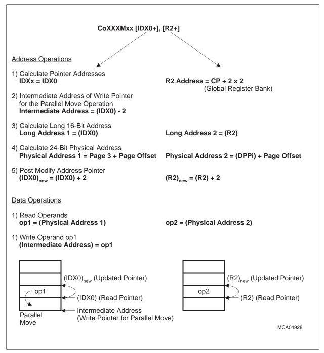
Figure 4-16 Arithmetic MAC Operations with Parallel Move
