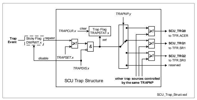
Figure 6-39 SCU Trap Structure
