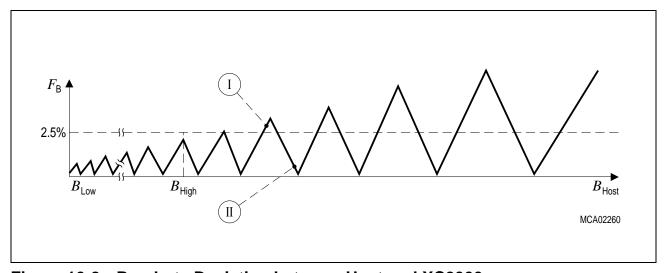
Figure 10-2 Baudrate Deviation between Host and XC2000
