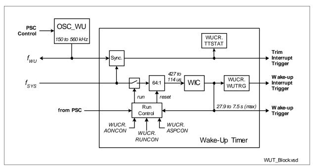
Figure 6-33 Wake-up Timer Logic
