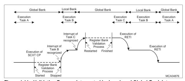
Figure 4-11 Validation Process Interrupted by Local- and Global-Bank Intr.
