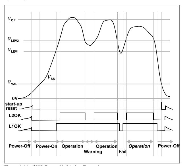
Figure 6-26 SWD Power Validation Example
