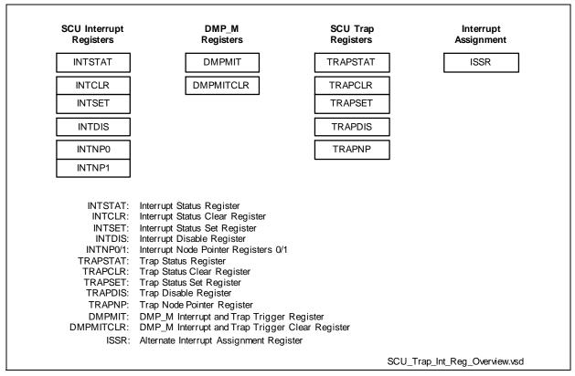
Figure 6-37 SCU Interrupt and Trap Register Overview
