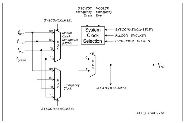
Figure 6-11 Clock Control Unit, SYSCLK Generation
