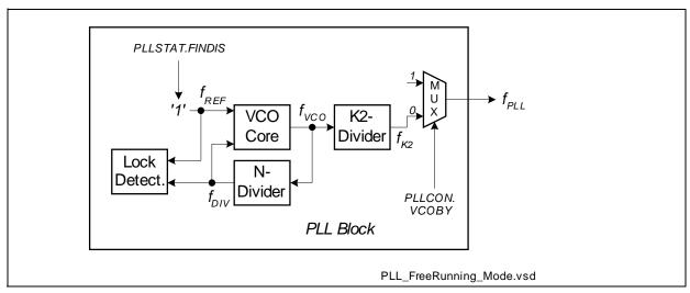
Figure 6-8 PLL Free-Running Mode Diagram
