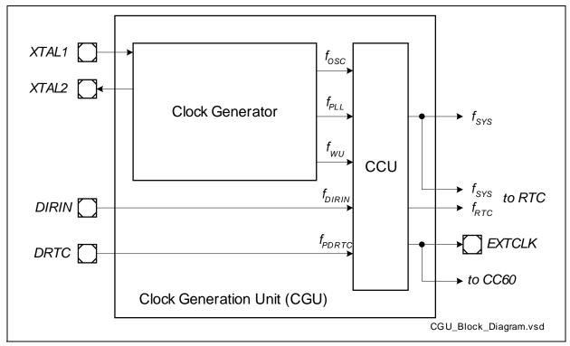
Figure 6-1 Clock Generation Unit Block Diagram
