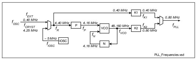
Figure 6-9 Overview on Frequency Ranges for the PLL Block
