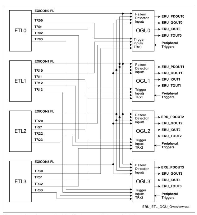
Figure 6-23 Connecting Matrix between ETLx and OGUy
