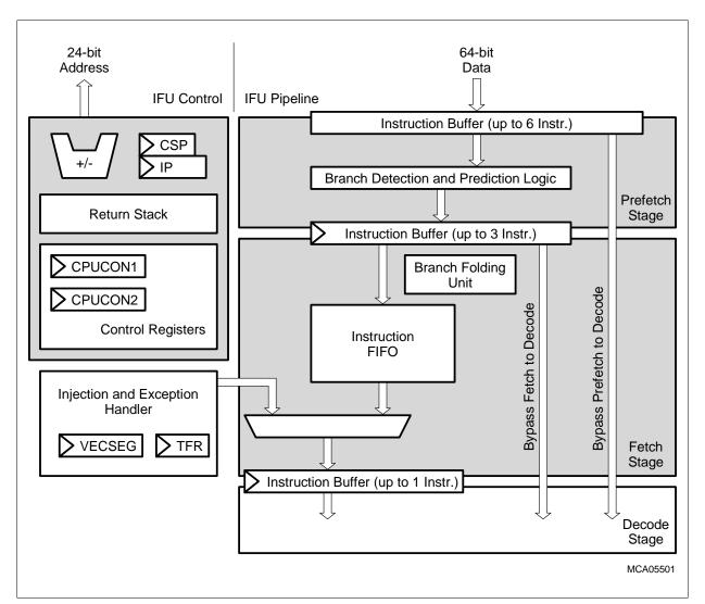
Figure 4-2 IFU Block Diagram
