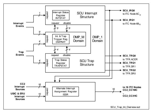
Figure 6-36 SCU Interrupt and Trap Overview
