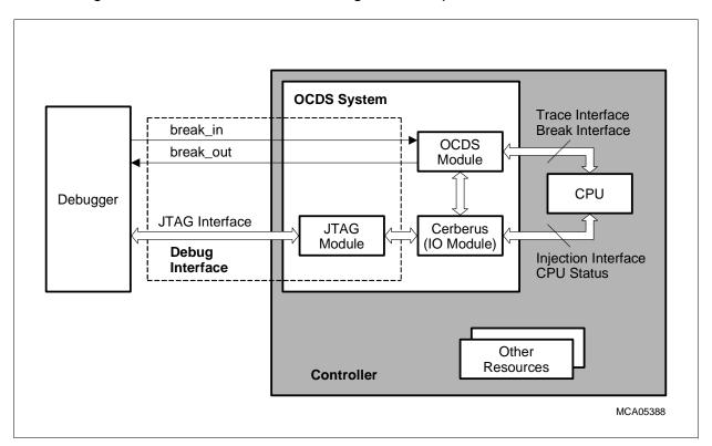
Figure 11-1 OCDS Overall Structure
