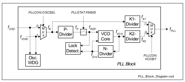
Figure 6-5 PLL Block Diagram
