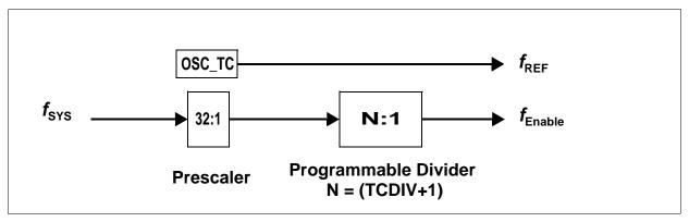
Figure 6-30 Temperature Compensation Clock Generation
