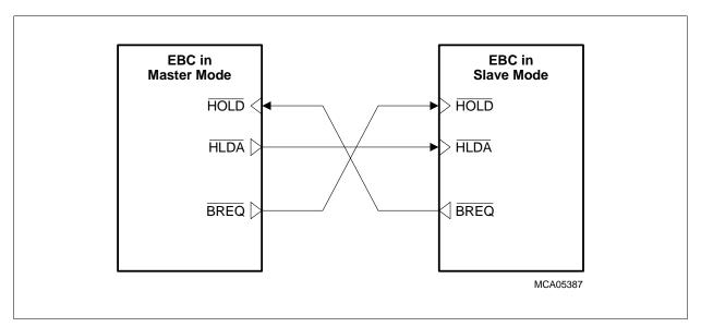
Figure 9-15 Connecting two XC2000 Using Master/Slave Arbitration
