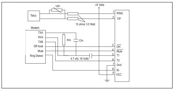
Rm and CM provide the impedance match with the telephone line. These values are country dependent. The chart below show the correct Rm and Cm values and correct XE10X0 model for various countries. VR1 provides protection from voltage surges on the telephone line. The table below show the recommended breakdown voltage for VR1.
