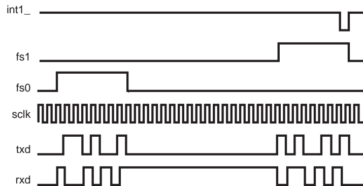
Figure 21. CODEC Interface Timing (8-Bit Mode)
