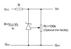
Figure 1: This circuit will allow the reference to be trimmed over a wide range. The device is specified over a  $\pm 5\%$  trim range.
