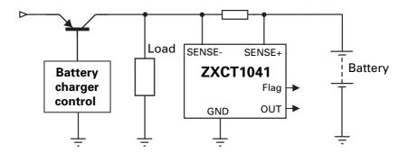
When choosing appropriate values for  $R_{\text{SENSE}}$  a compromise must be reached between in-line signal loss (including potential power dissipation effects) and small signal accuracy.
