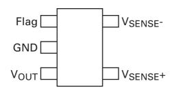
The very low offset voltage enables a typical accuracy of 2% for sense voltages of only 10mV, giving better tolerances for small sense resistors necessary at higher currents.
