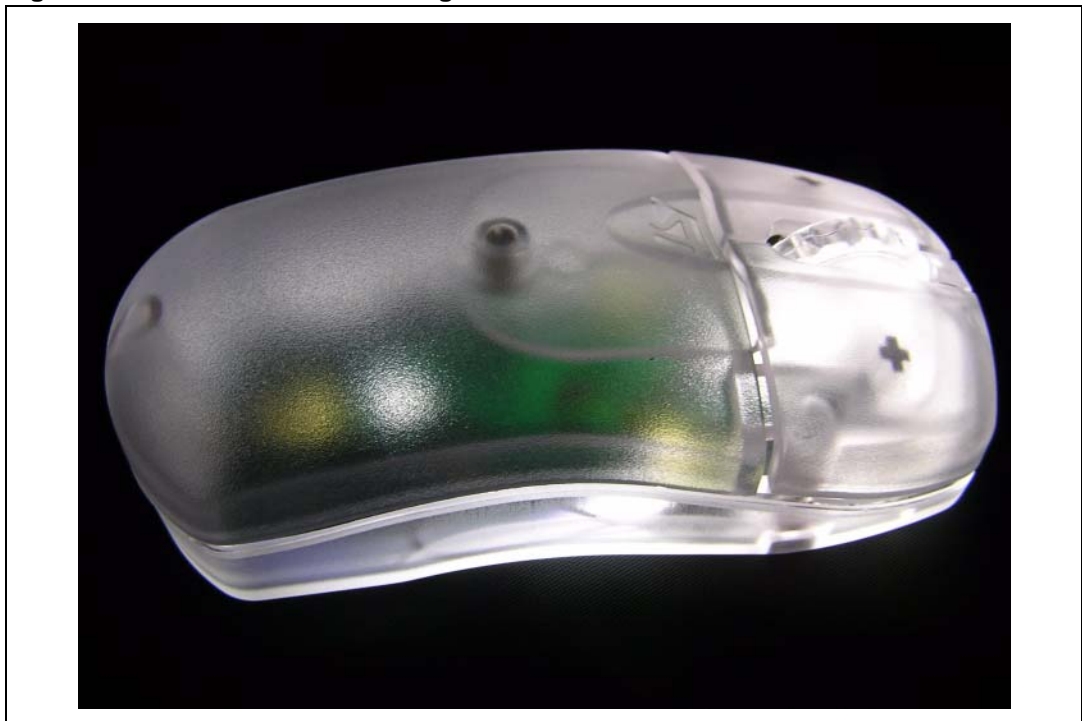
Figure 1. VT5365 reference design mouse
